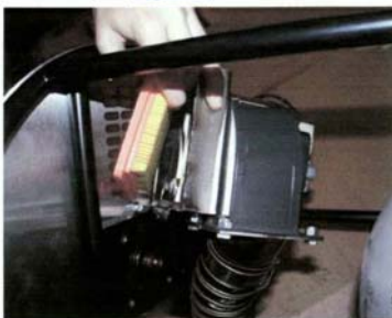
Figure 4. Filter Under Blower
