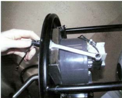
Figure 3. Removing the Blower
